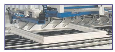
Profile margins, as well as technologically caused distortions to the welded sash, can be regulated effortlessly.
